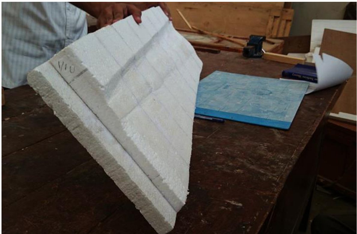
Figure 2. Polystyrene blocks were glued together to form a mold
